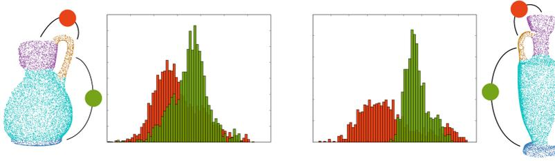
Fig. 3: **Comparison of spectral distances between two pairs of segments.** The distribution of the commute time distances between pairs of points on the base and the handle (green) and on the handle and the neck (red) are shown. Despite shape discrepancy, the histograms still capture the key features of the shape topology: The base is “farther away” to the handle than the neck.
