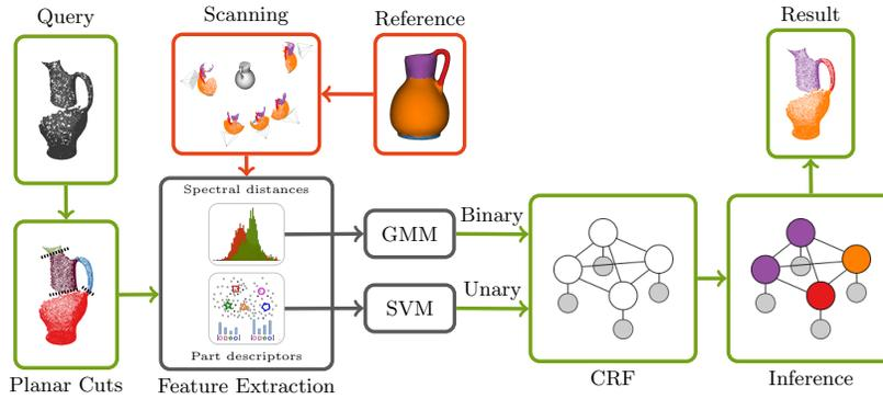
Fig. 1: Overview of our approach. A segmented mesh of the reference shape is used for training. The query is a point cloud of a similar partially observed shape.
