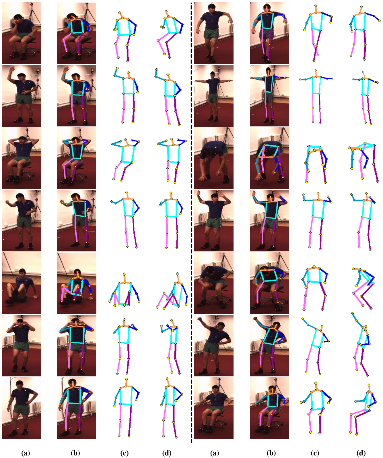
Figure 1: A few qualitative results from Human3.6M dataset [2]: (a) represents input images, (b) shows refined 2D poses while (c) and (d) correspond to estimated 3D poses from two different views.
