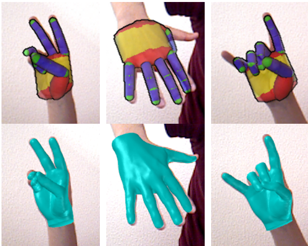
Fig. 14 Qualitative comparison with (Oikonomidis et al, 2011a). Each image pair corresponds to the pose estimate of the FORTH tracker (up) and our tracker (down)
