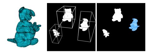
**Fig. 1. From left to right:** *a)* 3D model of object. *b)* Potential bounded subsets of the search space. *c)* Projection of the mesh. The pose is correctly estimated.
